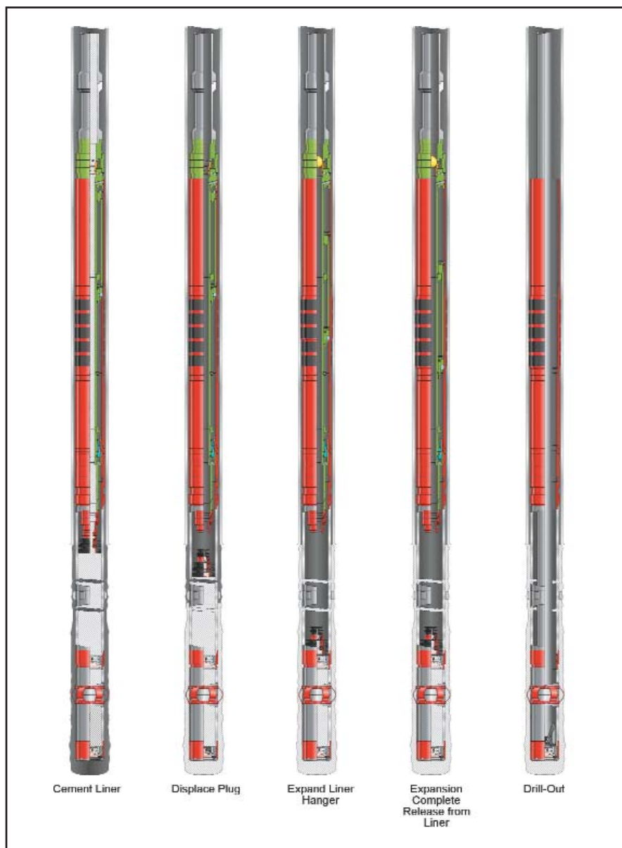
Figure 7. VersaFlex liner hanger system running.
